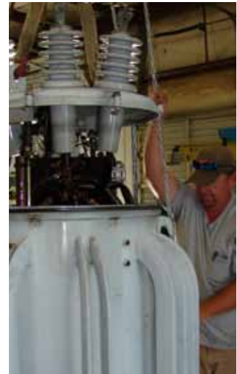
Shop Disassembly of a Regulator
